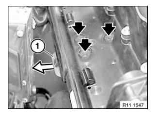
Remove sealing cap (1) in direction of arrow. Remove seal plugs (arrowed) upwards.
