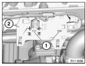
Unclip both retaining tabs through openings (1) and remove retaining plate (2) in upward direction.
