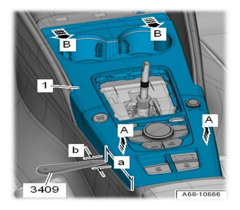
Remove this panel with an integrated MMI control unit. Loosen this control unit together with the chromed frame of the shift lever.
