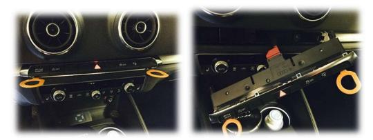
Removing the button strip: Use the standard release clips
