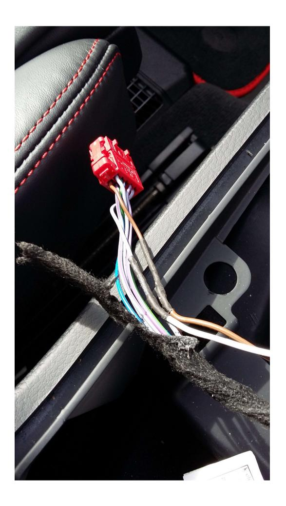
6. Route the cable set into the passenger footwell, To do this, simply dismantle the climate control part and / or the push button bar.
