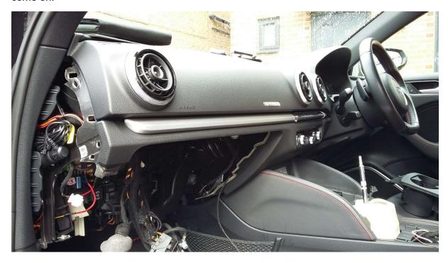
2. Disassemble the centre console. For this purpose the use of the centre console has to be expanded. Lever the leather of the gearshift knob upwards. Pull the trim panel A upwards and unplug it. Pull the panel B backwards.
