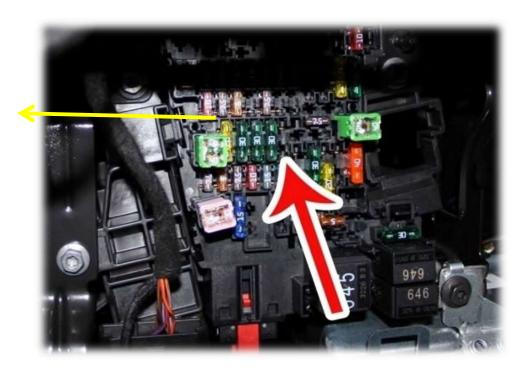
If there is no free slot (depending on the existing vehicle equipment), please install a new secure slot or solder the cable to an existing line. The other cable set must be routed along the spout into the engine compartment. Open the bonnet.
