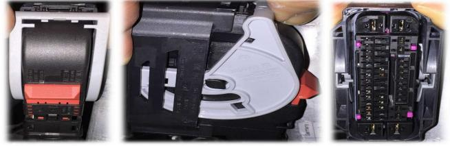
10. Install the cables to the ABS control unit when installing the plug in the ABS control unit, ensure that the lock is correct. This plug must be 100% unlocked - by moving the red insert down this will allow you to move the grey lever down and remove the plug. Disconnect the connector and remove it from the control unit.
