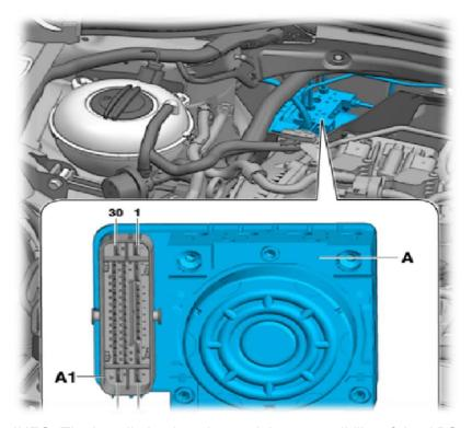
INFO: The installation location and the accessibility of the ABS control unit vary according to the motor installed.
